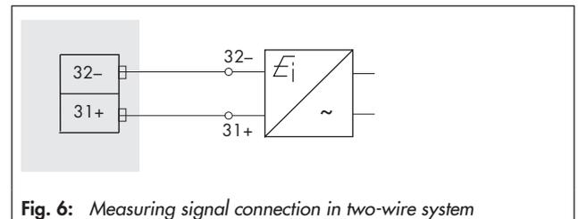
A Media 5 device can be fitted upon delivery with a 4 to 20 mA current output. A retrofit in already installed devices (even former device model from 2001 onwards) is possible on site.
